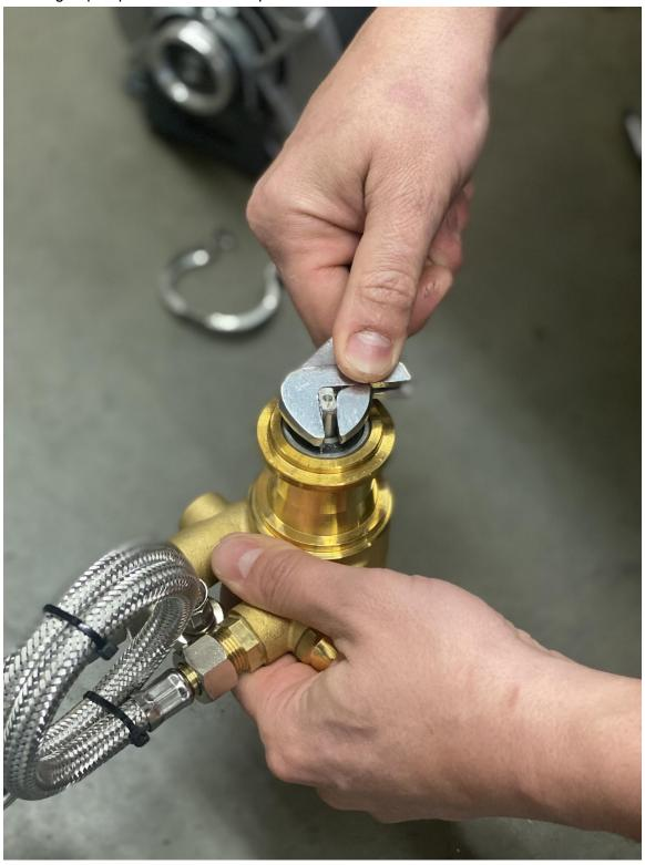
Do the same test with the new pump head. Our Mavam pump heads complete with all the fittings in place but you still need to lubricate the shaft that connects to the inside of the motor. Use an all purpose lubricant or grease.
