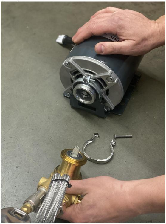
If the motor is turning proceed to testing the pump head. Spin the shaft with a wrench to test how much force is required to make the internals move. If it's a struggle to turn you indeed have a damaged pump head and must replace.
