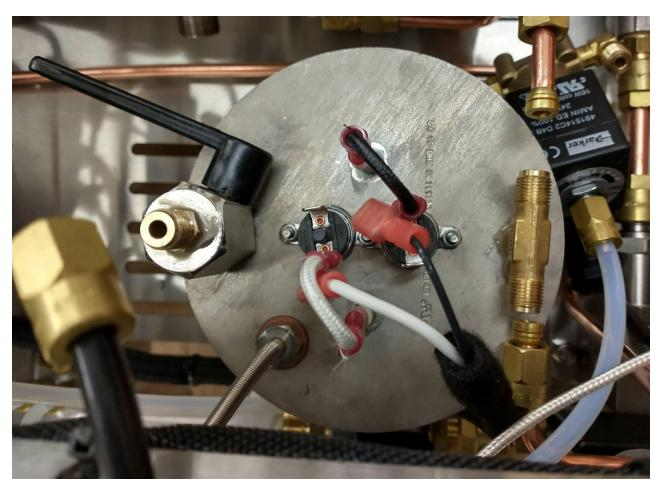
5. Remove both brass 6mm nuts on the tee fitting. \*Note: there is a 1mm flow restrictor on the cold water input side, the section of the tee pointing directly at you or to the front of
