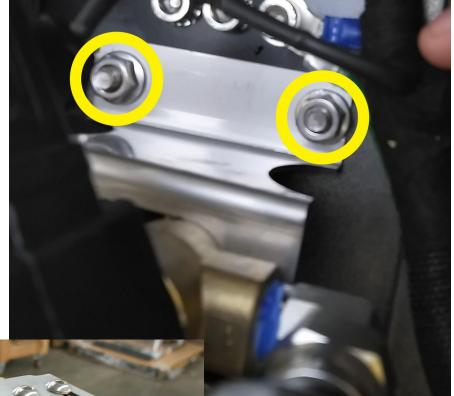
\*Mach 2: First, you will need to remove the top cover and cup tray and then disconnect the brass 6mm nut from the wand's side and brass 8mm nut, 14mm wrench, from the copper tubing connection only on the valve.
