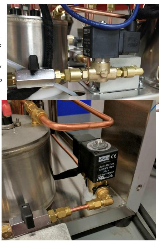
3. Unscrew the autofill boot and save the rubber gasket & screw for reinstalling. \*Note: Handle with care these wires are fragile and cannot be near any water that may leak out. If water does leak out, clean up with a towel before continuing.
