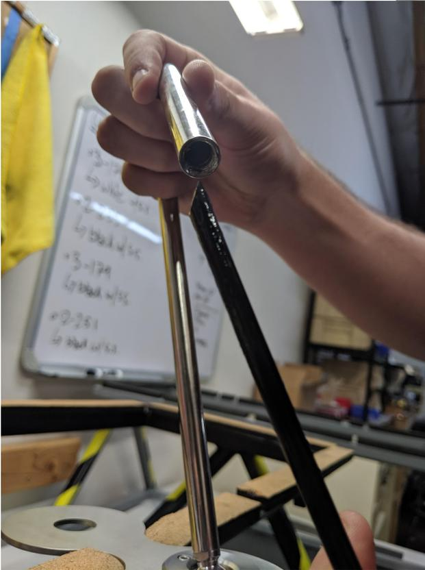
5. Proceed to slowly push the tubing, with food safe lubricant, into the side of the steam wand with the steam wand tip. **\*Note: Be sure to push slowly and in small increments, keeping your hand no more than 2 to 3 inches front the metal steam wand edge. Do not bend or kink the tubing, this would ruin the process and cause damage.**
