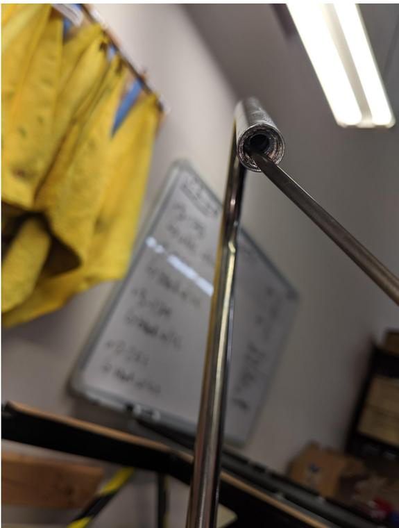
4. Apply food safe lubricant to the exterior of the new black teflon tubing. About the first 2 inches down from one of the ends. This is what will be inserted first.
