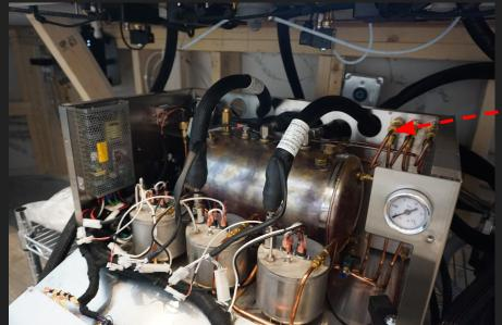
Hoses connected to boilers- center to center, right to right. Shut offs open.
