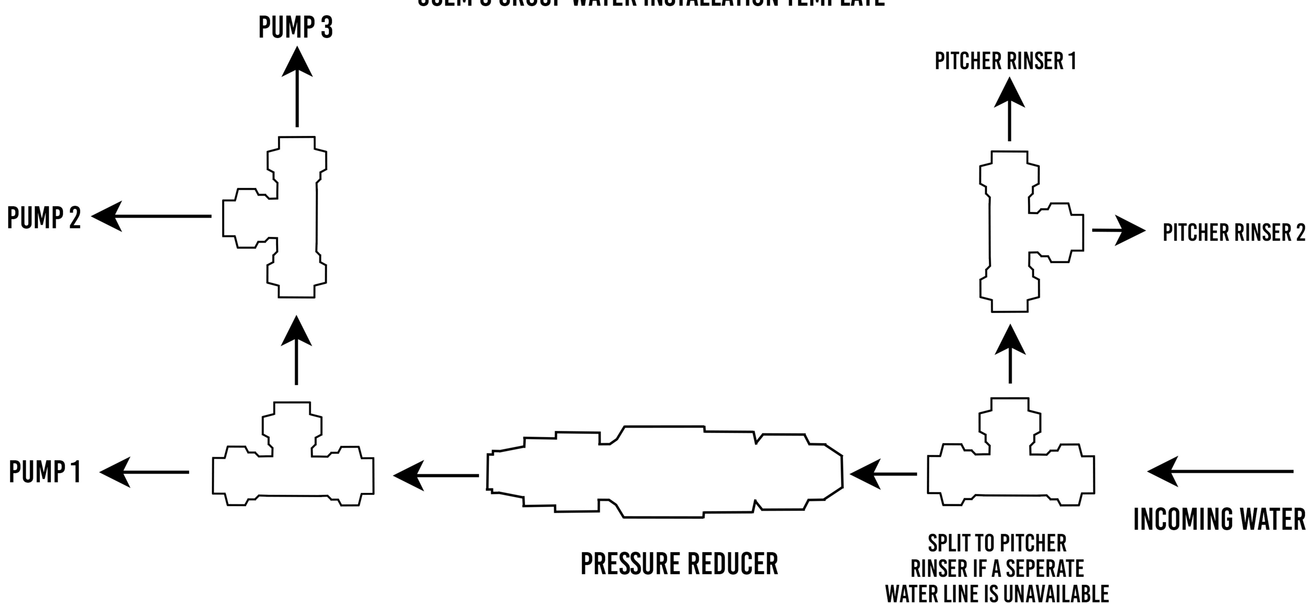
THE PRESSURE REDUCER PLACEMENT IS VERY IMPORTANT, WITHOUT IT PRE-INFUSION WILL NOT FUNCTION AS INTENDED
