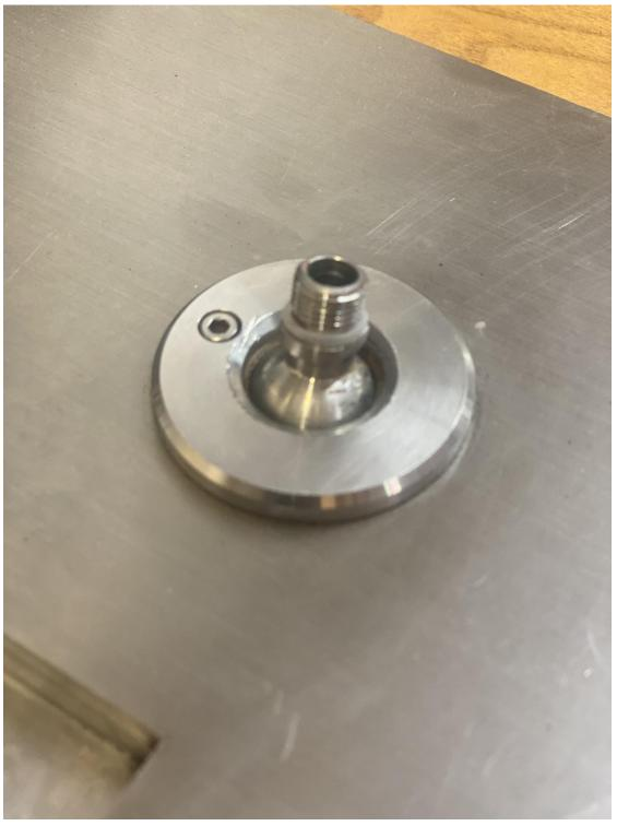
Install the new wand on the ball and tighten very tight to make a solid seal. The clear o'ring might shear off which is ok, as it is adding to the seal.
