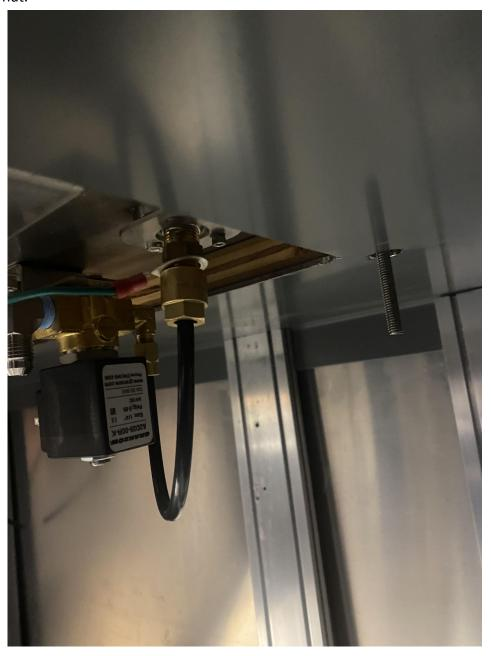
Install the 1" or 30mm tube into the steam wand tip then test the steam wand and check for leaks.
