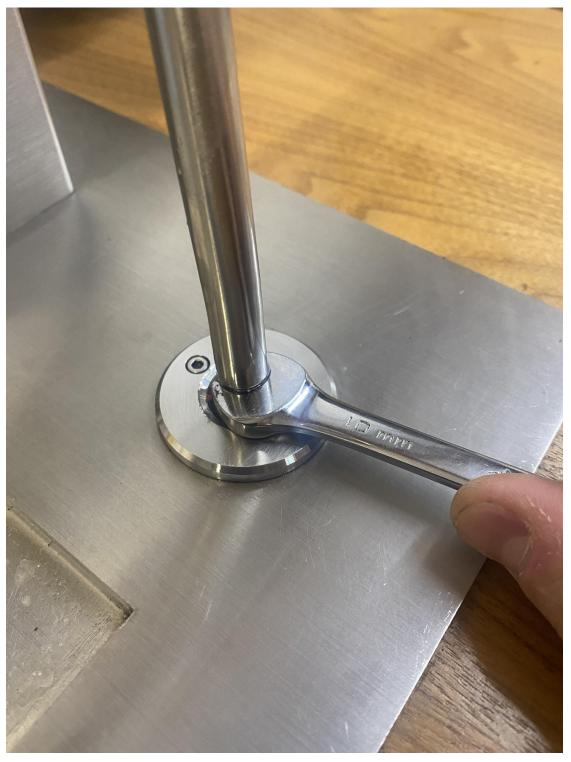
The wand ships with red lock tight but add more to the ball if needed and install the clear o'ring on the ball fitting as shown
