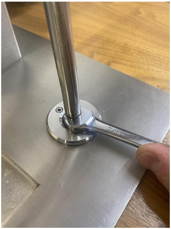
We recommend removing the ¼ brass fitting and teflon taping and / or using red loctite on the threads going into the ball joint to make sure a steam tight seal is achieved.
